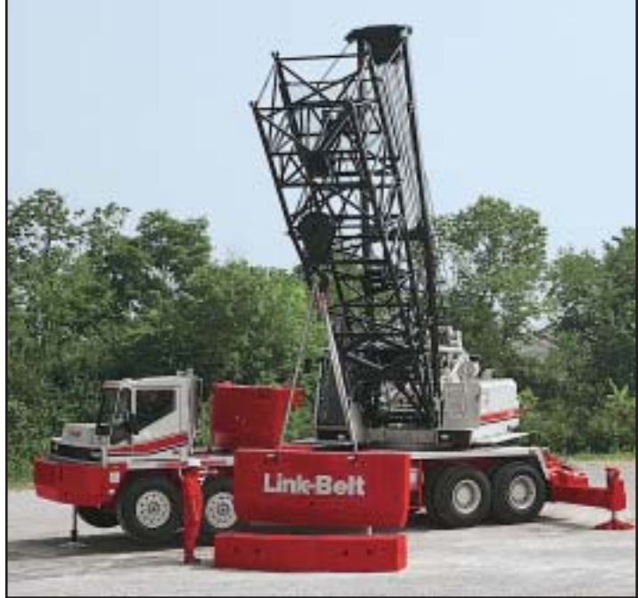
Hydraulic cylinders pull/extend bottom pins and rear outrigger box is simply slipped off of hooks.
