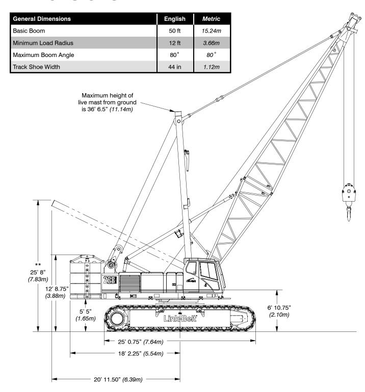
Note: \*\* @ Maximum boom angle (80°) with maximum boom [260 ft (79.25m)], maximum rotation radius occurs.
