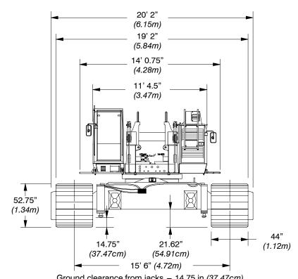
Ground clearance from jacks - 14.75 in (37.47cm) Ground clearance from frame - 21.62 in (54.91cm)
