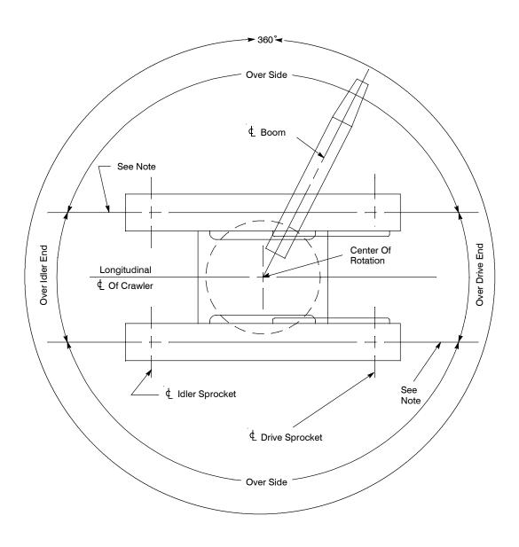
$\textbf{Note:} \ \ \textbf{These Lines Determine The Limiting Position Of Any Load For Operation Within Working Areas Indicated}.$
