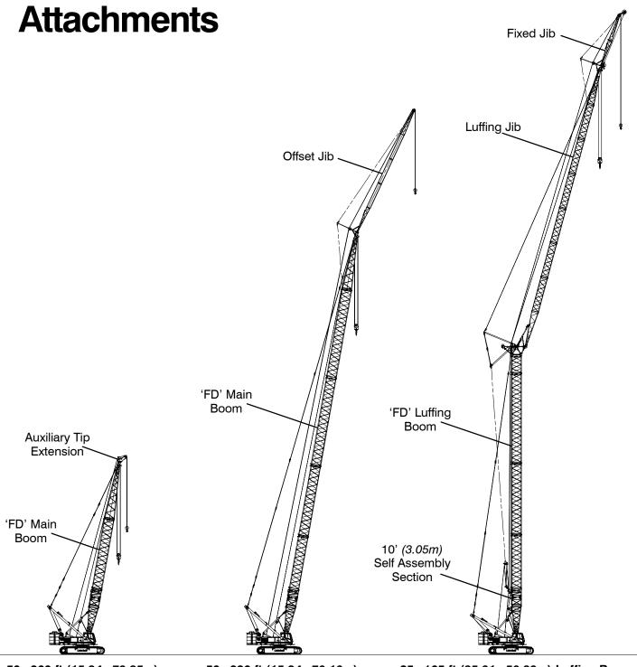
50-260 ft (15.24-79.25m) Main Boom With 5 ft (1.5m) Tip Extension 50-230 ft (15.24-70.10m) Main Boom With 30-75 ft (9.14-22.86m) Offset Jib 85-165 ft (25.91-50.29m) Luffing Boom + 80-160 ft (24.38-48.77m) Luffing Jib With 30 ft (9.14m) Fixed Jib
