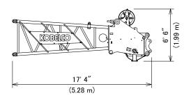
Taper Insert Boom Weight: 1,190 lbs (540 kg) includes cable roller.
