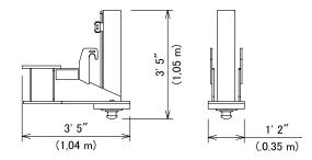
Gantry with Lower Spreader Weight: 5,560 lbs (2,520 kg)
