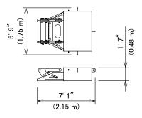
Counterweight Self-Removal Cylinder Weight: 3,700 lbs (1,680 kg)
