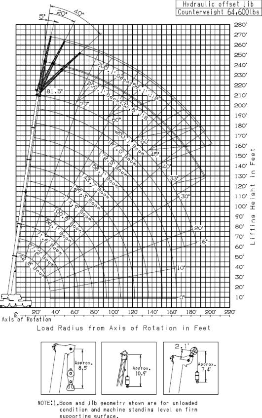
supporting surface. Boom deflection and subsequent radius and boom angle change must be accounted for when applying load to hook.
