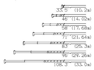
NOTE: Load radiuses for jib operation are given for reference with the boom fully extended to 108.3' (33m).
