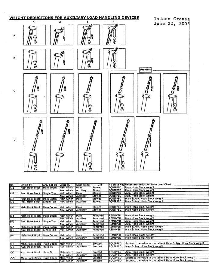
EQUIPPED Aux. Hook Block Top Jib Aux. winch Auxiliary Erected Main & Aux. Hook Block weight EQUIPPED EQUIPPED EQUIPPED EQUIPPED Aux. Hook Block weight Main winch | Main Erected Aux. Hook Block Top Jib Aux. Hook Block weight
