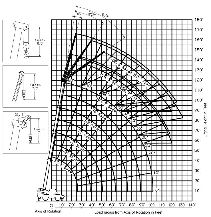
**NOTE:** Boom and jib geometry shown are for unloaded condition and machine standing level on firm supporting surface. Boom deflection and subsequent radius and boom angle change must be accounted for when applying load to hook.
