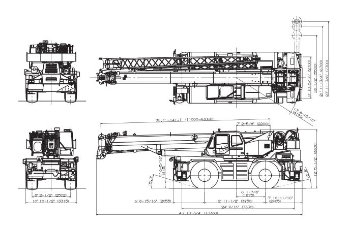
Note: Dimension is with boom angle at -1.6 degree.
