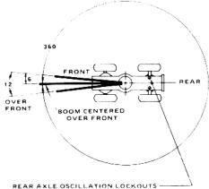
REAR AXLE OSCILLATION LOCKOUTS -MUST BE SET TO MAINTAIN 360 CAPACITIES.
