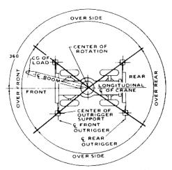
NOTE BOLD LINES DETERMINE THE LIMITING POSITION OF ANY LOAD FOR OPERATION WITHIN WORKING AREAS INDICATED.
